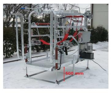
Hydraulic lift up to 50 cm enabling work in an upright position while hoof trimming front legs
