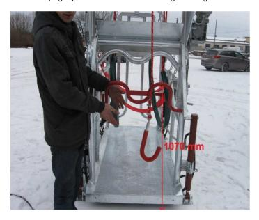
A unique back gate enabling work in in an upright position
