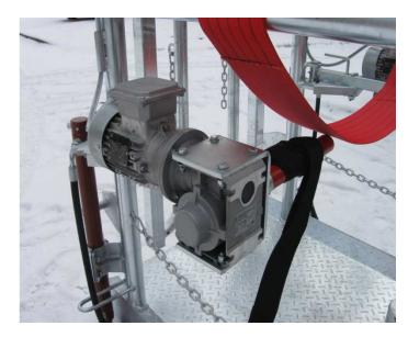
✓ Electric front and back leg lifts by means of German-made geared motors
